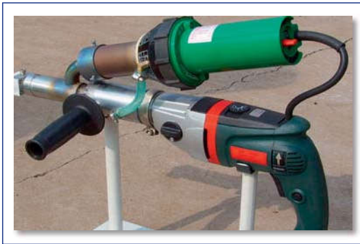
▶ Extrusion Plastic Welding
